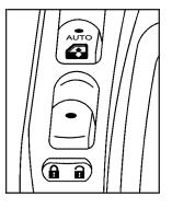
The window switches are located on each side of the shift lever on the center console.
